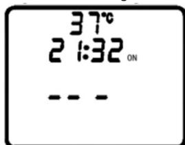
Figure 7: Pre-heating is turned on
